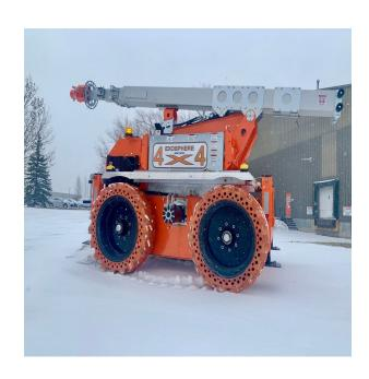
The Exosphere Anchor Systems 4x4 All Terrain features a 4 stage 38-foot mast. Up to two (2) independent 92 (2336 mm) offset Arm Anchors for the attachment of a personal fall arrest system (PFAS).
